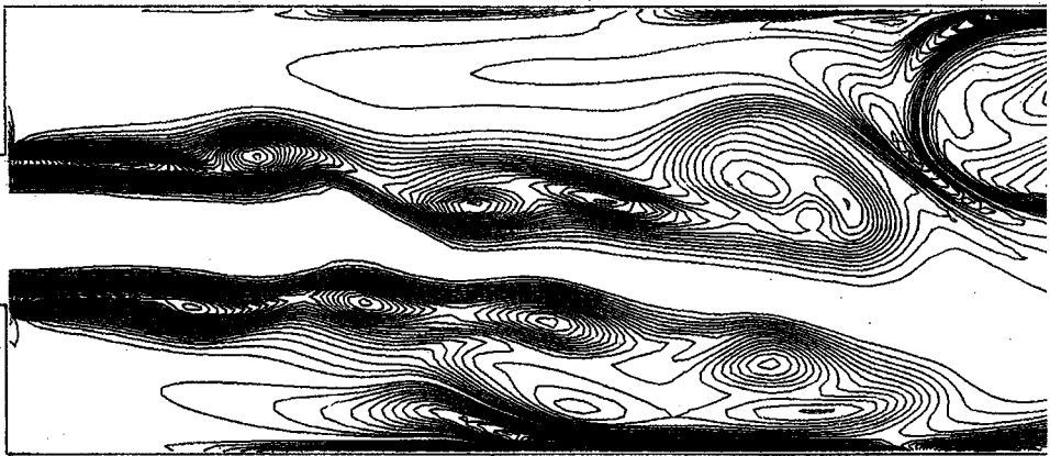
Figure 2. Unsteady subsonic two-dimensional flow in the channel with sudden expansion.
